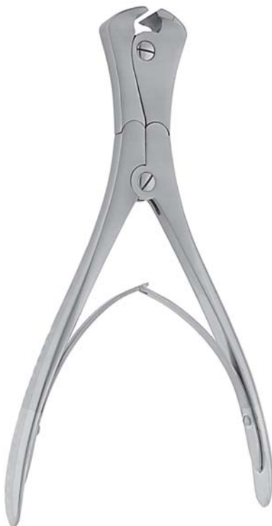
7436 Wire Cutter 220 mm TC soft wire 2.5 mm hard wire 2.2 mm
