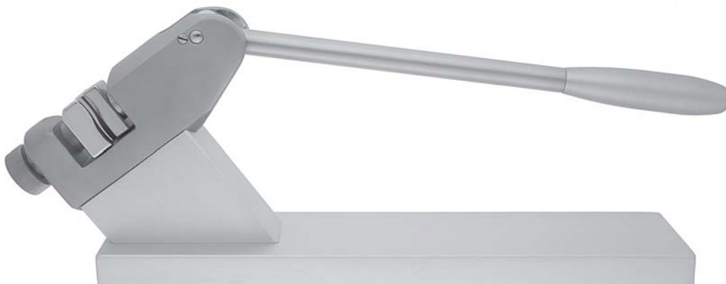
9420 Bending Device to bend straight and angled plates
